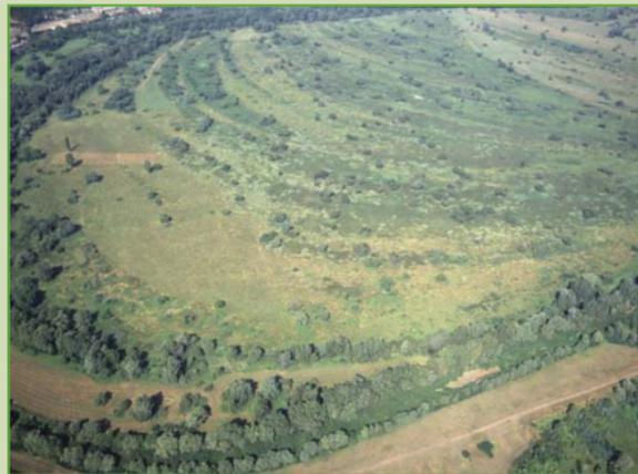
Regular water supply of the marshes was cut off in the middle of the 19th century as a result of river regulation works. After the works were finished, the new and old dams of the Tisza River became connected and a structure, called „ring dam” by the locals, was formed that completely cut off water supply from the rivers to the area.
